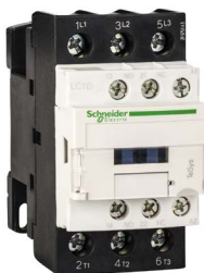
Schneider Contactor 18A 7.5kW, 3 Pole, 3 Normally Open Main Contacts, Auxiliary Contacts 1 N/O & 1 N/C
